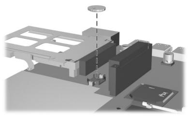
Removing the RTC Battery
